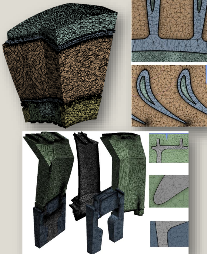
CFD Mesh Creation for Nozzle Block and Rotor Blade
