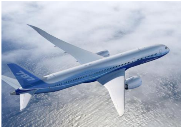
Boeing 787-8 “more electric airplane” with many conventional systems converted to electric power
