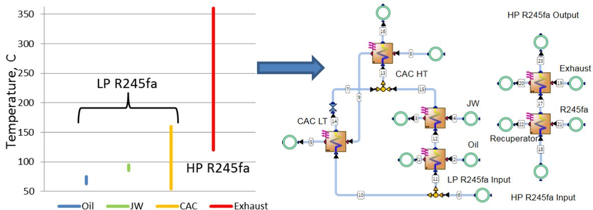
**Figure 2:** The distribution of heat flows according to their temperatures and the option of their utilization (where LP and HP – low pressure and high pressure; LT and HT – low temperature and high temperature; CAC – charge air cooler)
