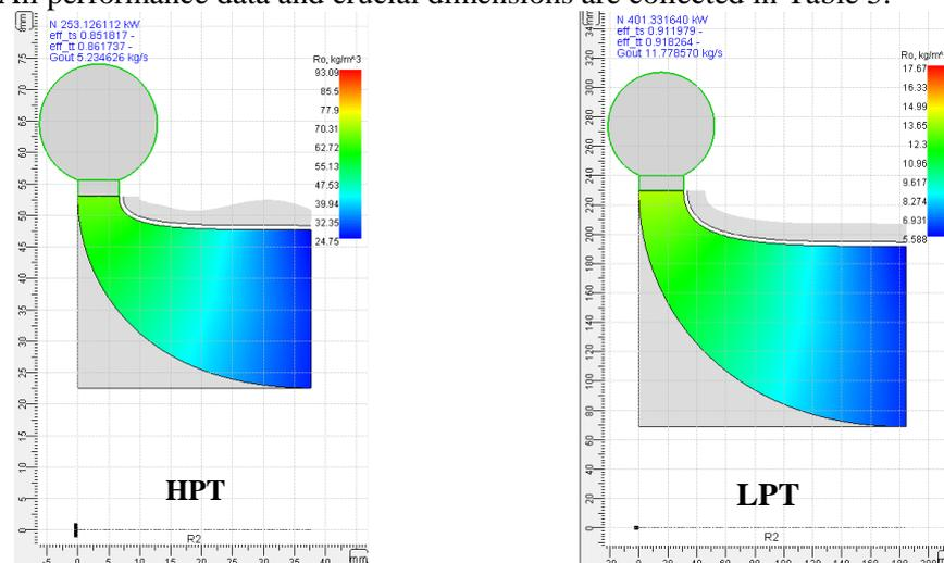
Figure 8: Turbines meridional view with density field
