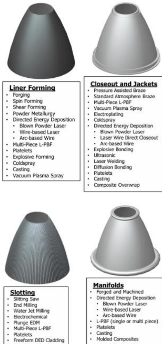
Figure 19: Various manufacturing technologies considered for channel wall nozzle fabrication (CWNF) [8]
