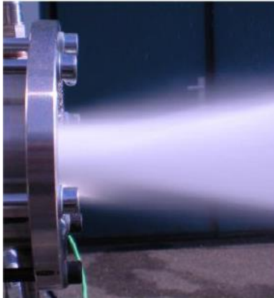
Figure 17: 30 bar hot-run of an integrated CMC thrust chamber assembly including ceramic injector. [15]
