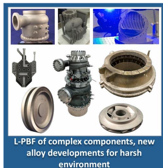
Figure 16: Example applications produced with AM method Laser powder bed fusion (L-PBF). [16]
