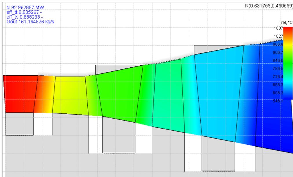
Furthermore, AxSLICE allows us to modify each single airfoil slice geometry directly without going back to the 3D CAD optimizing stator and rotor blades profile on the row-by-row results.
