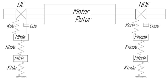
**Fig. 3 – Rotor-Bearing System with Supports (Calculation Scheme)**
