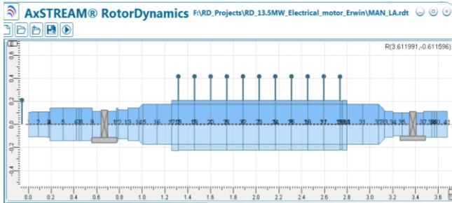
Fig.5 – Rotor Dynamics FE model
