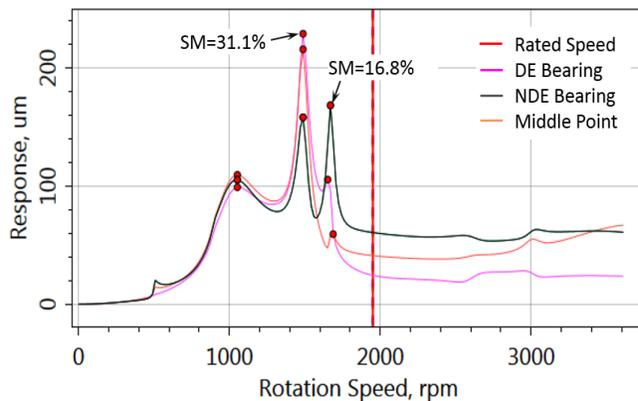
**Fig. 11 – Frequency Response Characteristics for Optimized Rotor-Bearing System Design**
