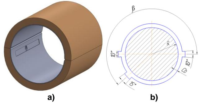
**Fig.2 – Induction Motor DE Bearing CAD Model (a) and Varying Parameters Scheme (b)**
