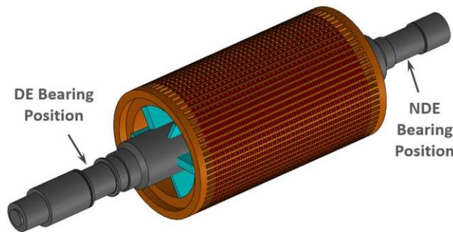
**Fig.1 – Induction Motor Model**
