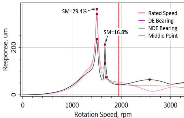
Fig. 6 – Frequency Response Characteristics for Initial Rotor-Bearing System Design
