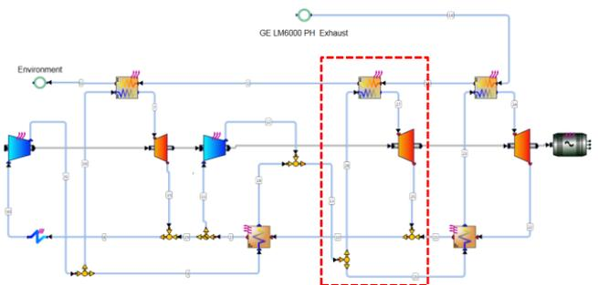
Fig. 9 Composite bottoming Cycle 3 scheme
