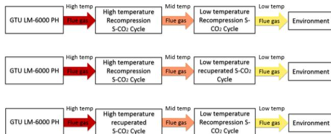
Fig. 1 Some examples of bottoming S-CO<sub>2</sub> cycles combinations
