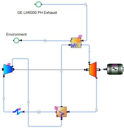
Fig. 13 Recuperated S-CO<sub>2</sub> bottoming cycle scheme (Cycle 7)
