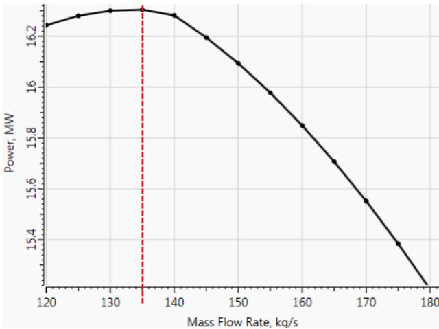
Fig. 3 Total power of the bottoming cycles vs. mass flow rate in the recompression cycle
