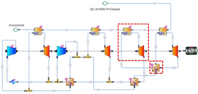
Fig. 10 Composite bottoming Cycle 4 scheme
