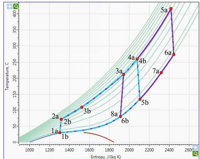
Fig. 5 Recompression and recuperated cycles processes diagram in TS coordinates
