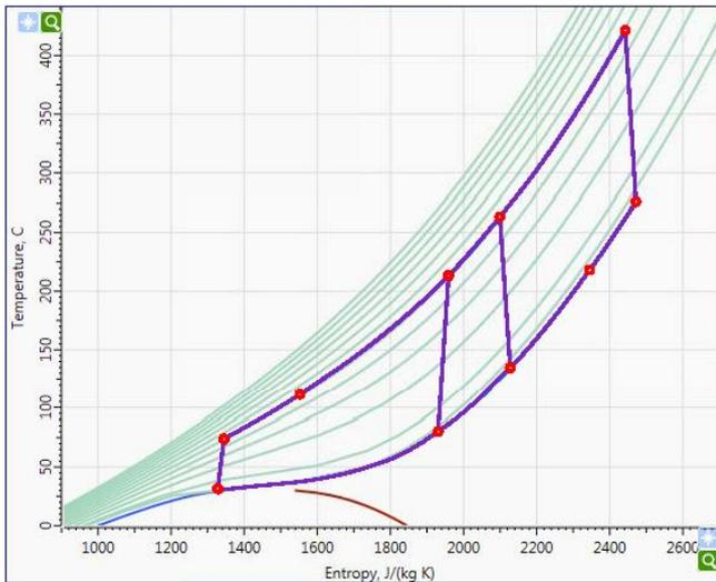
Fig. 7 Composite recompression-recuperated bottoming cycle processes in TS diagram
