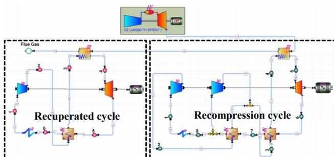
Fig. 2 Combination of recompression S-CO<sub>2</sub> cycle and recuperated S-CO<sub>2</sub>
