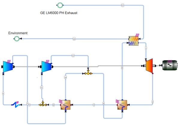
Fig. 12 Recompression S-CO<sub>2</sub> bottoming cycle scheme (Cycle 6)
