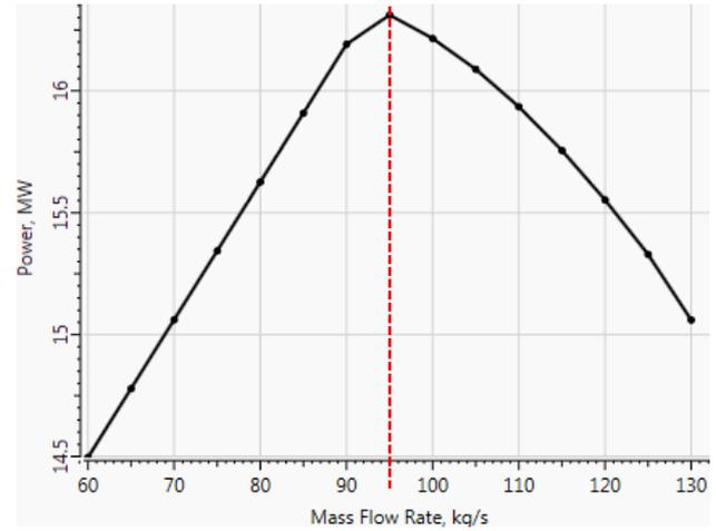
Fig. 4 Total power of the bottoming cycles vs. mass flow rate in the recuperated cycle
