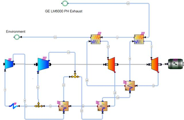
Fig. 11 Recompression bottoming cycle with reheat scheme (Cycle 5)
