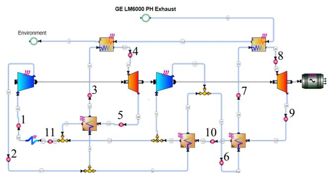
Fig. 6 Composite recompression-recuperated bottoming cycle
